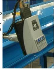
form 3 individual manufacturers were being used and this provided its own problems to the support staff. Each scanning point also used an automated "Kit ID" scanner to identify the kit to Banta Global Turnkey's own internal Production Monitoring Software System and also an "Employee Badge" scanner to provide accountability.
