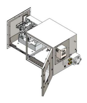
Enclosure: 316L stainless steel, 2 mm thickness
