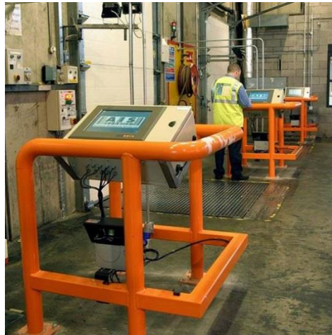
AIS Automatic pallet scanning stations at Diageo's shipping bays
