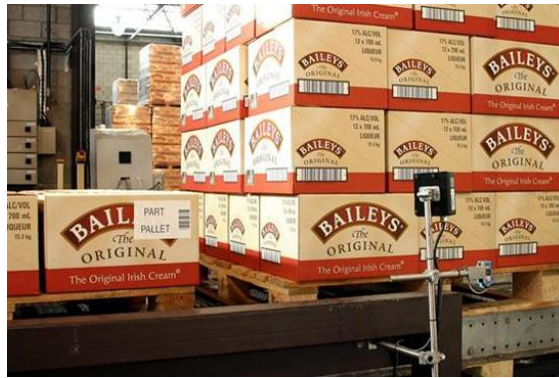
Datalogic DS4600 scans pallets before shrink wrap
