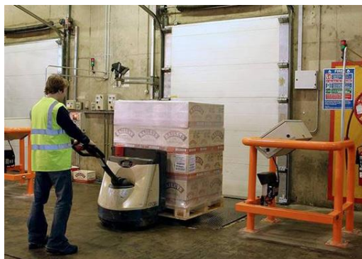
Pallet scanned at dispatch bay by automatic scanning station
