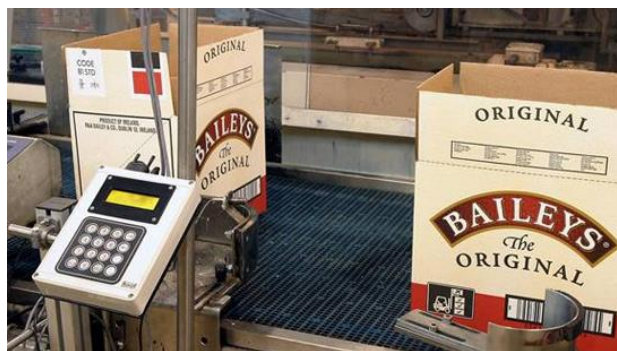
AIS VPM2 Data entry terminal mounted in the Diageo Bottling Hall
