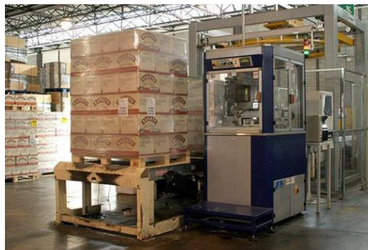
ALTech pallet label applicator automatically labels two adjacent sides of pallet
