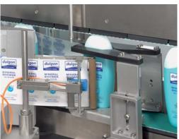
Preparing the labelling process by separating, aligning and stabilizing the products.
