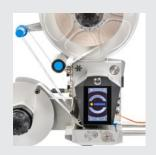
For automatic label detection the FS03 sensor of HERMA senses the last label on the peel plate, thereby ensuring maximum precision.
