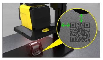
**Reading DPM codes on electronics parts**
