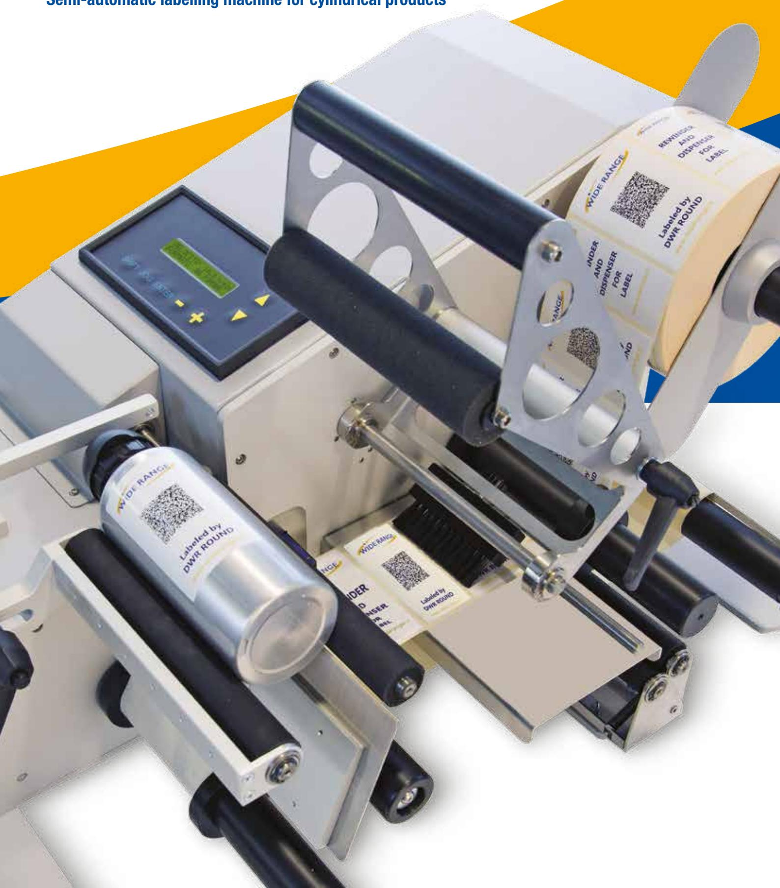
**DWR ROUND** is a semi-automatic labelling machine for the application of self-adhesive labels to cylindrical products.
