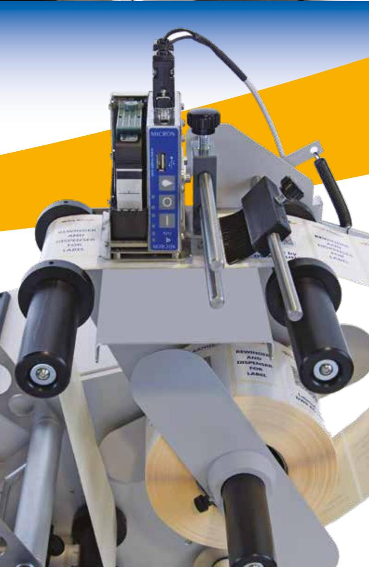
DWR ROUND can apply wraparound or front/back labels, even of different dimensions positioned on the same reel.
