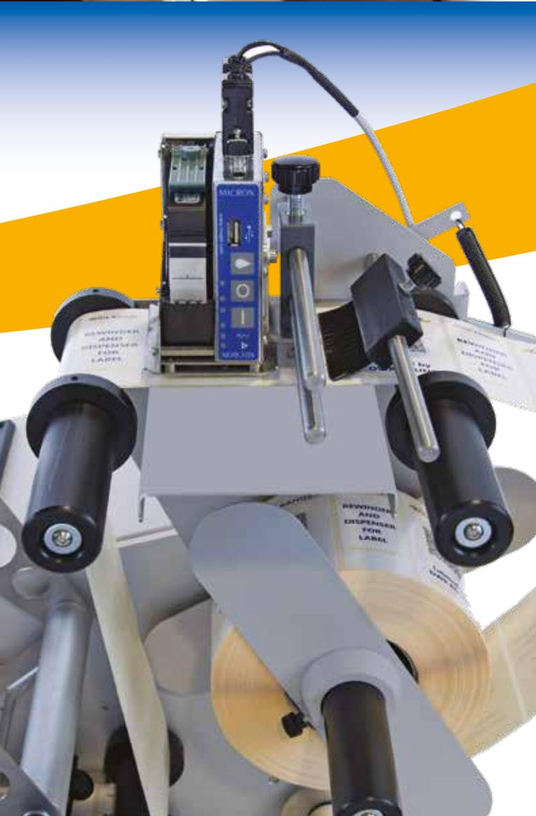
DWR ROUND can also be equipped with an inkjet marker with HP technology for printing variable data such as date and time, barcodes and text with a maximum height of 12.7 mm, a resolution of 300 dpi and speed synchronised with the label supply speed.
