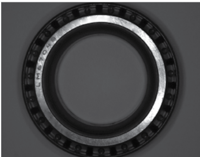
Without HDR: Embedded parts are unclear.
