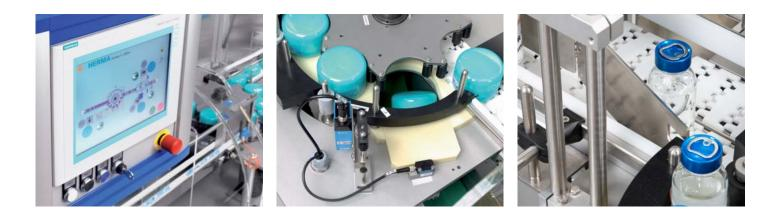
Simple machine operation with the help of a clearly laid out and easyto-use touch panel. Among the optional functions are units for dispensing faulty labels or rejecting incorrectly labelled products.
