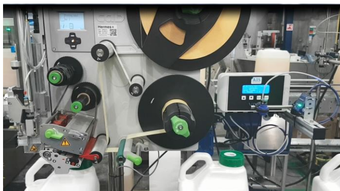
Cab Hermes + system applying label. Checked by Matrix 210 and VB5.
