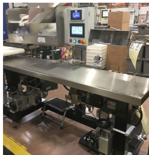
Label is inspected by the Datalogic Matrix 210 and the AIS VB6.
