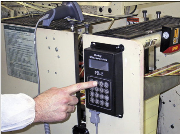
ORBY VB2 in action featuring keyboard entry of the bar code to be verified by the fixed mount scanner. The ORBY eliminates the requirement for an expensive and bulky PC or PLC in the vicinity.
