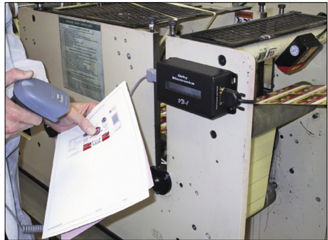
ORBY VB1 in action, verifying bar codes on a Mark Andy 8 color label press. The ORBY allows the operators to rapidly, safely, and securely change the bar code to be verified.
